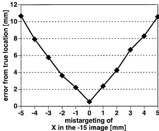
**Figure 14.** Line graph illustrates the discrepancy between true and calculated location with a targeting error of  $-5$  to  $+5$  mm in the x coordinate on the  $-15^\circ$  image. The graph assumes accurate targeting on the  $+15^\circ$  image and with respect to y.
