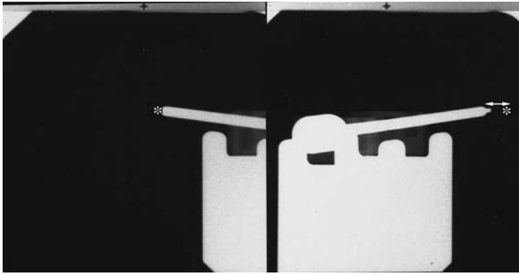
**Figure 13.** Stereo radiographs show a targeting error (bias) of 3 mm along the x axis on the  $+15^\circ$  image (horizontal line) with no error on the  $-15^\circ$  image.
