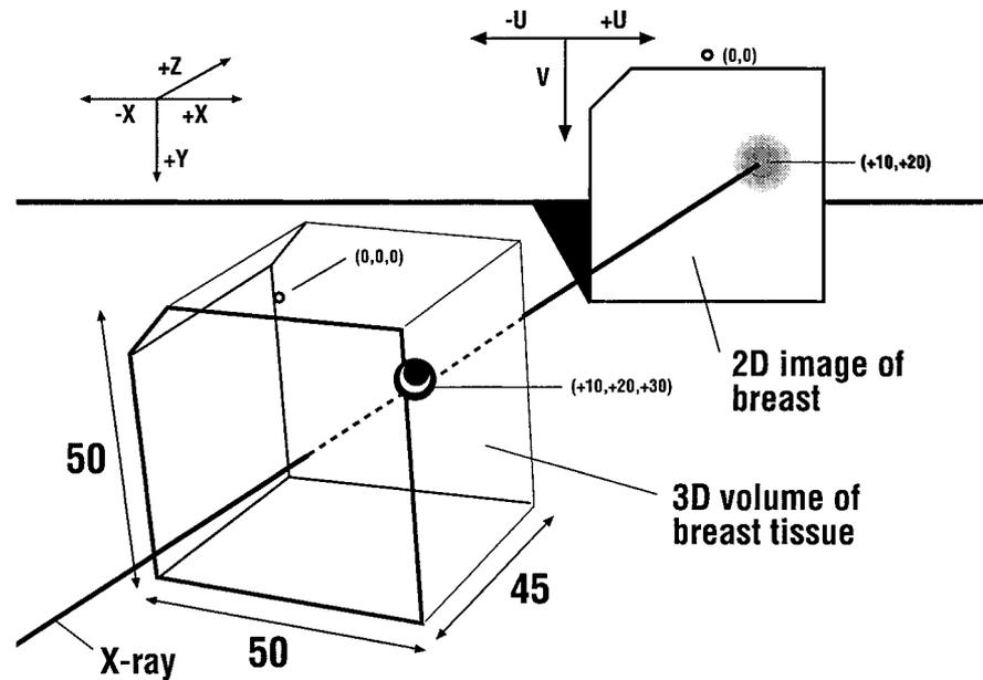
**Figure 1.** Diagram illustrates the relationship between a 3D object ( $x$ ,  $y$ , and  $z$  coordinates) and a 2D image ( $u$ ,  $v$  coordinates).
