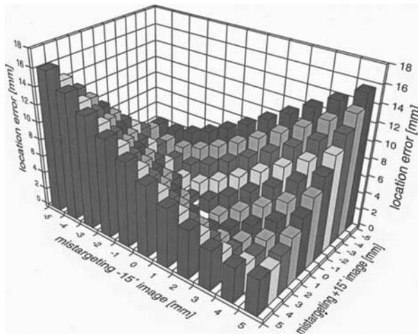
**Figure 18.** Three-dimensional bar graph illustrates localization error (in millimeters) with targeting errors on both stereo images.
