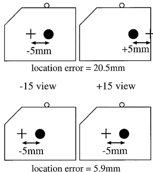
**Figure 17.** Diagram shows how depth calculation can be markedly altered if the targeting errors are in opposite directions.
