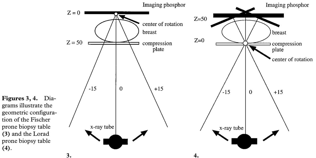
**Figures 3, 4.** Diagrams illustrate the geometric configuration of the Fischer prone biopsy table (3) and the Lorad prone biopsy table (4).
