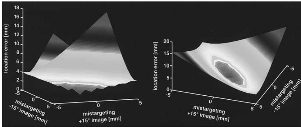
**Figure 19.** Radiograph illustrates surface display of theoretic error created with all combinations of errors in x targeting on one or both stereo images.
