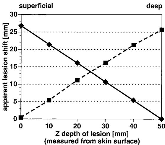
**Figure 6.** Graph illustrates the relationship between parallax shift (as measured on +15° and -15° images) and depth z (cf Fig 5). With the Fischer system (solid line), parallax shift increases as a lesion is located more superficially. With the Lorad system (dashed line), parallax shift increases with increasing lesion depth. This difference results from the different placement of the center of rotation on the two units.
