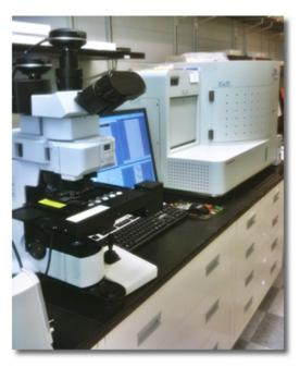
The microscope (above, left) is part of the Olympus VS110 workstation, which includes high resolution monitor (center), and the attached NanoZoomer slide scanner (far right), which can process up to 210 slides at a time in each slide cassette.
